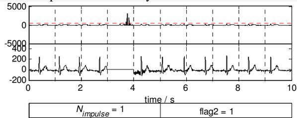
Figure 3. The ECG with huge impulse (upper panel) and ECG removing huge impulse (lower panel).
